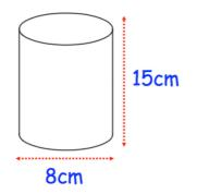
The cylinder is made from titanium. The density of titanium is 4.43g/cm<sup>3</sup>
