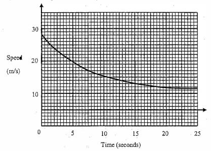
Use the graph to estimate the distance travelled by the car in the first 20 seconds.
